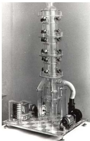
Fig. 2. Model and industrial absorber is set at the Kherson plant
