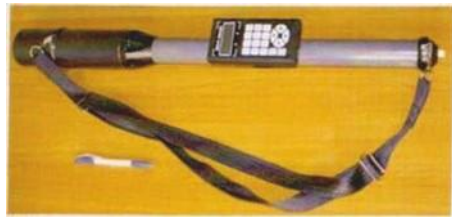
Fig. 3.5 MKS-01 Sovetnik. (From: Gurachevsky 2010) method of monitoring contamination for gamma-emitting radionuclides. The monitoring needs to be conducted using a robust and
