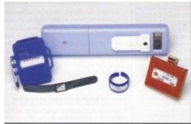
Fig. 3.4 Different types of pocket dosimeters. (From: Gurachevsky 2010)
