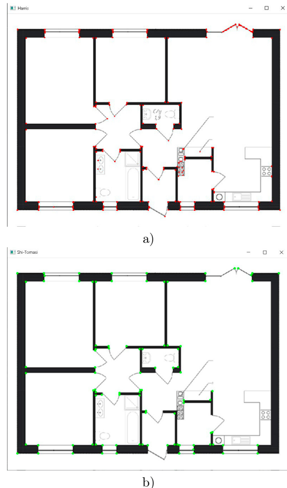
FIG. 5. (color online) Recognizing of Harris and Shi–Tomasi detectors estimated number of angles: the Harris (a) and Shi–Tomazi (b) detector test images.
