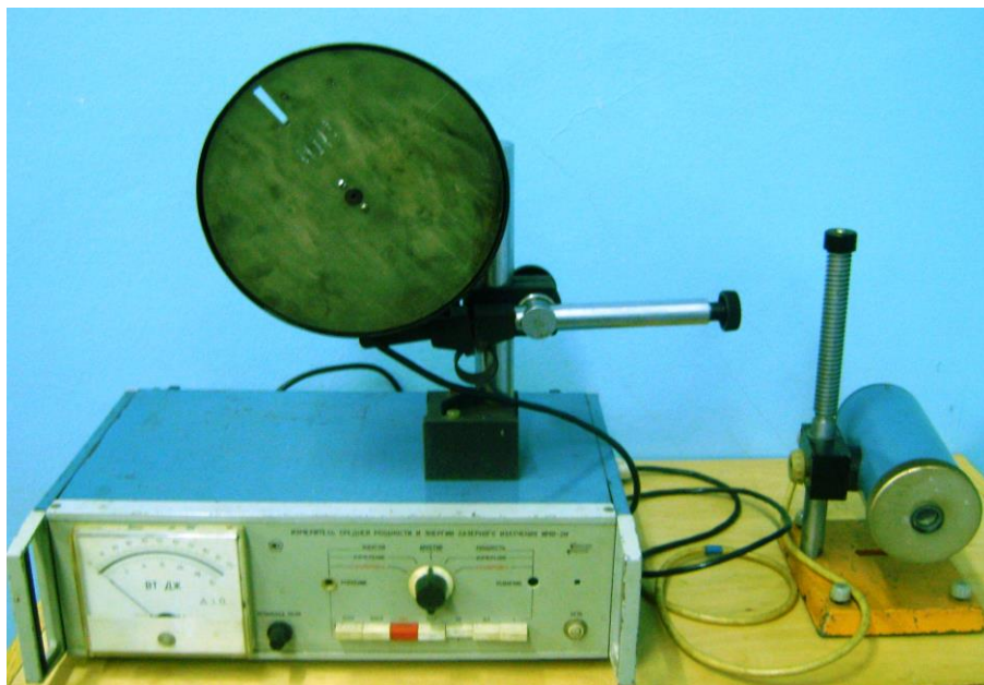
Figure 2.1 – Meter for average power and energy pulses of laser radiation IMO – 2H
