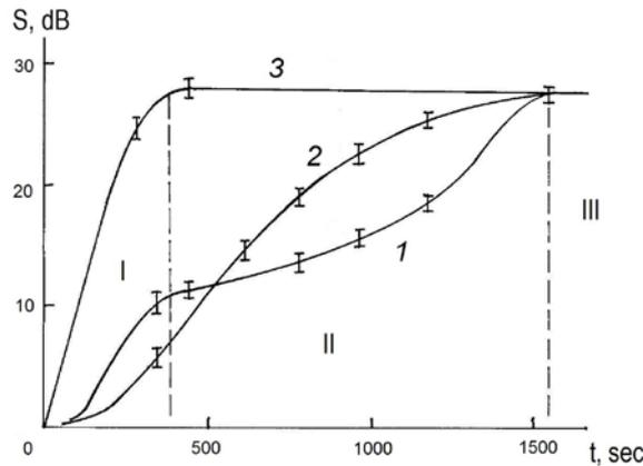
**Figure 2.** Microwave radiation energy attenuation by thawing ice on the base of: **1** and **2** distilled and running water, **3** – 1% NaCl solution
