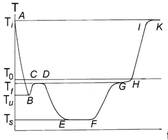
**Figure 3.** Kinetic dependence of PVA solution temperature at freezing-thawing. Temperatures:  $T_i$  – initial,  $T_0 = 0\text{ }^\circ\text{C}$ ,  $T_f$  and  $T_u$  – of freezing and overcooling solution,  $T_s$  – of a frozen sample exposure [7]
