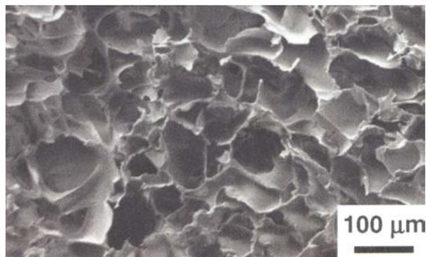
**Figure 5.** Surface structure of cryogel sample formed at  $T = -12\text{ }^\circ\text{C}$  from 10% mass concentration PVA water solution.
