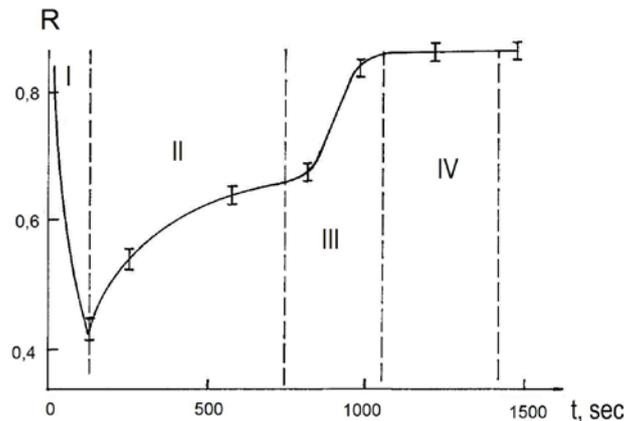
**Figure 1.** Changes of reflection coefficient of ice in the process of thawing. Microwave radiation frequency,  $\nu = 10$  GHz
