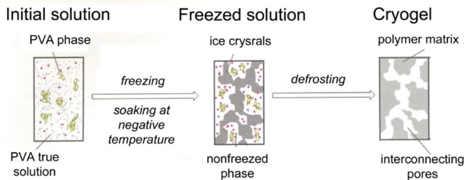
**Figure 4.** Scheme of cryotrope gelation [14]
