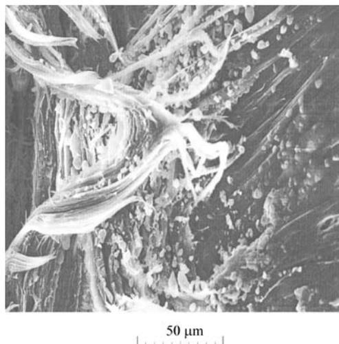
**Figure 9.** PVA (10 %) water cryogel structure modified by Seignette salt and filled in with active carbon (1.5 % mass.)
