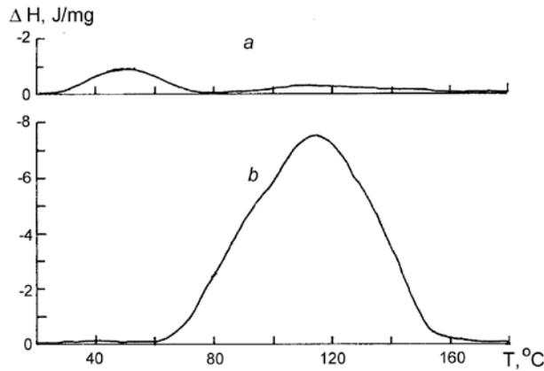
**Figure 8.** DSC curves of hydrogel (a) and obtained from it by threefold freezing-thawing cryogel (b)
