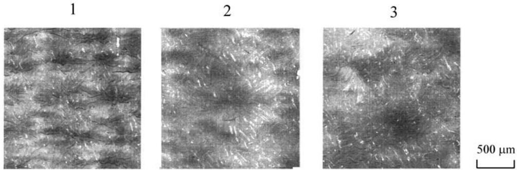
**Figure 7.** Surface structure (a) and IR spectra (b) of gel samples: **1** – original gel, **2** and **3** – cryogels obtained from it by means of single and twofold freezing
