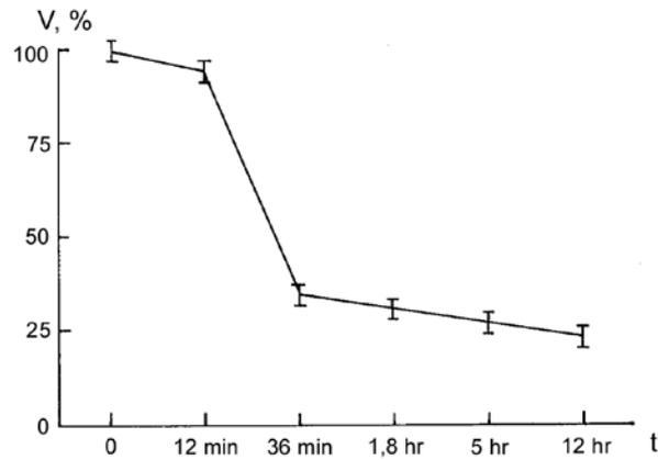
**Figure 6.** Volume dependence of 10% PVA solution hydrogel sample on thermostating time at  $T = 12^\circ\text{C}$  [14]
