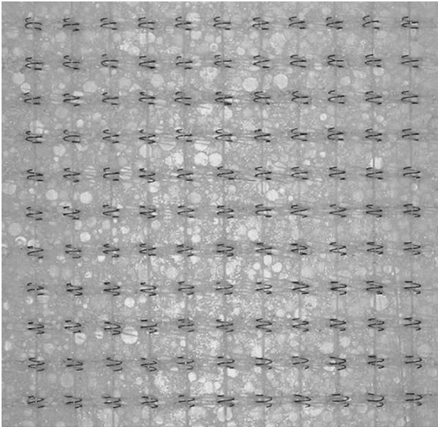
**Fig. 3.** Two-dimensional gyrotropic array composed of double-turn helical radiators fastened on a Styrofoam plate.
