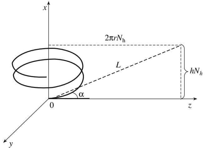
Fig. 1. Helix and the schematic view of its unraveled form.
