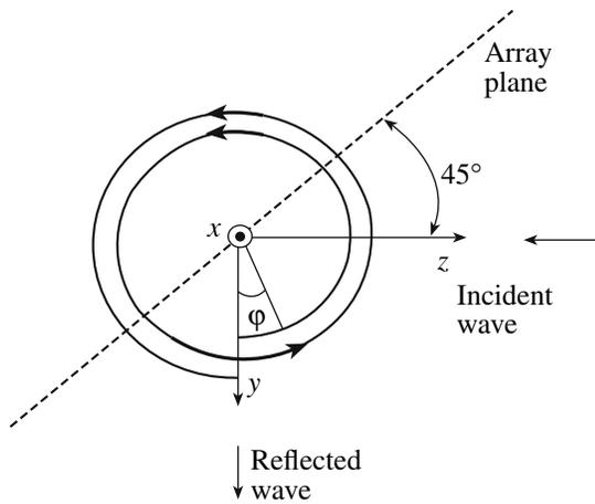
**Fig. 2.** Current distribution over a double-turn helix. The arrows show the current direction, with the current strength being proportional to the arrow length, and  $\varphi$  is the polar angle.
