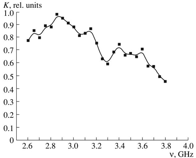
**Fig. 4.** Axial ratio  $K$  of the reflected wave vs. frequency  $\nu$  of the incident linearly polarized wave.
