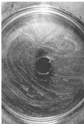
Fig. 10.6. Oriented Ps cell growth on an agar culture medium in a MF generated by a magnetoplastic cylindrical sample: axial magnetization B_r = 2.6 mT
