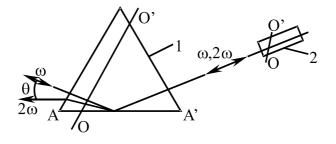
Using of a crystal CaCO<sub>3</sub> is caused by a significant anisotropy and tranparence of a crystal. The phase synchronism of interacting waves in a nonlinear crystal is carried out by moving of a prism 1 toward an optical axis OO'. The peak efficiency of transformation in created optical system makes  $\sim 80\%$ , that allows to use such type of the schemes in laser systems.
